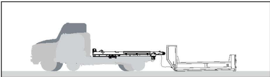
**Step 7—** Unhook the cable hook from the truck body and attach the hook at the hoist system's rear mounting bracket labeled Stow Hook Here.
