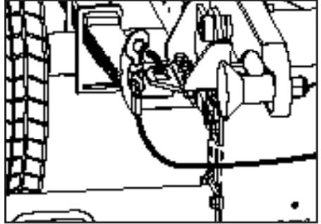
**Step 9—** If needed, press the button marked winch cable "IN" while keeping slight tension on the cable with your hands to prevent the cable from dragging on the ground. Always wear protective gloves when handling the winch cable.
